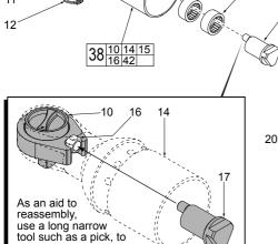
properly position the drive bushing (16) in the slot of the yoke (10). Align bushing so the end of the crankshaft (17) can be inserted into the drive bushing.
