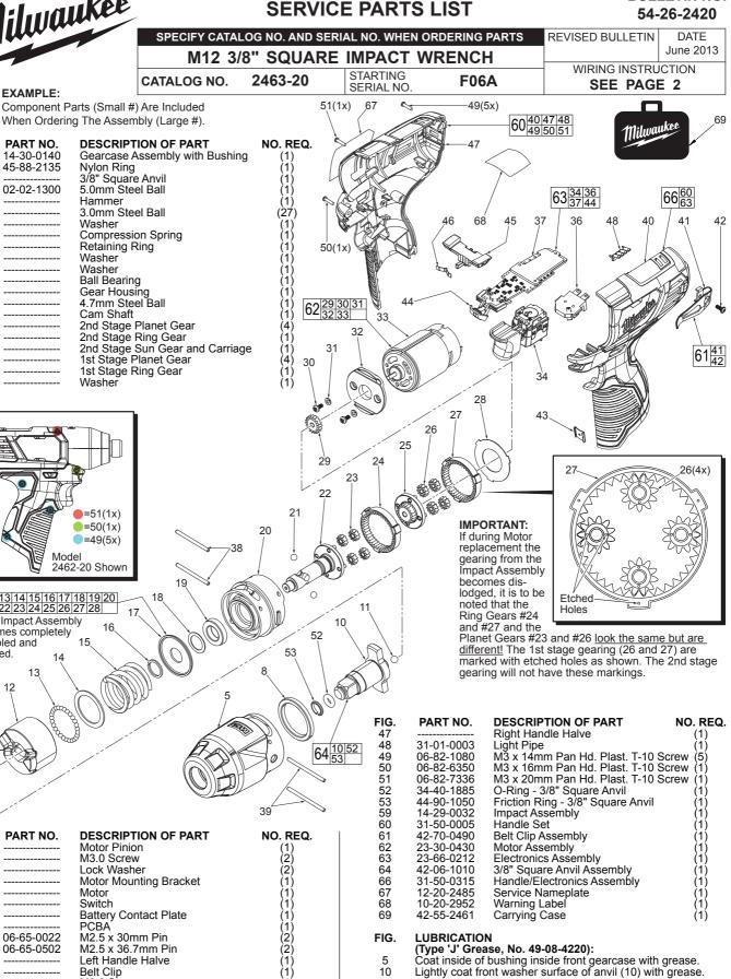
Coat pinion of motor assembly (62) with grease.
